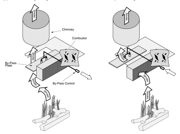
An optional combustor temperature probe is available from your dealer. It allows you to monitor the combustor temperature, which light off if the temperature is above 600° F.
